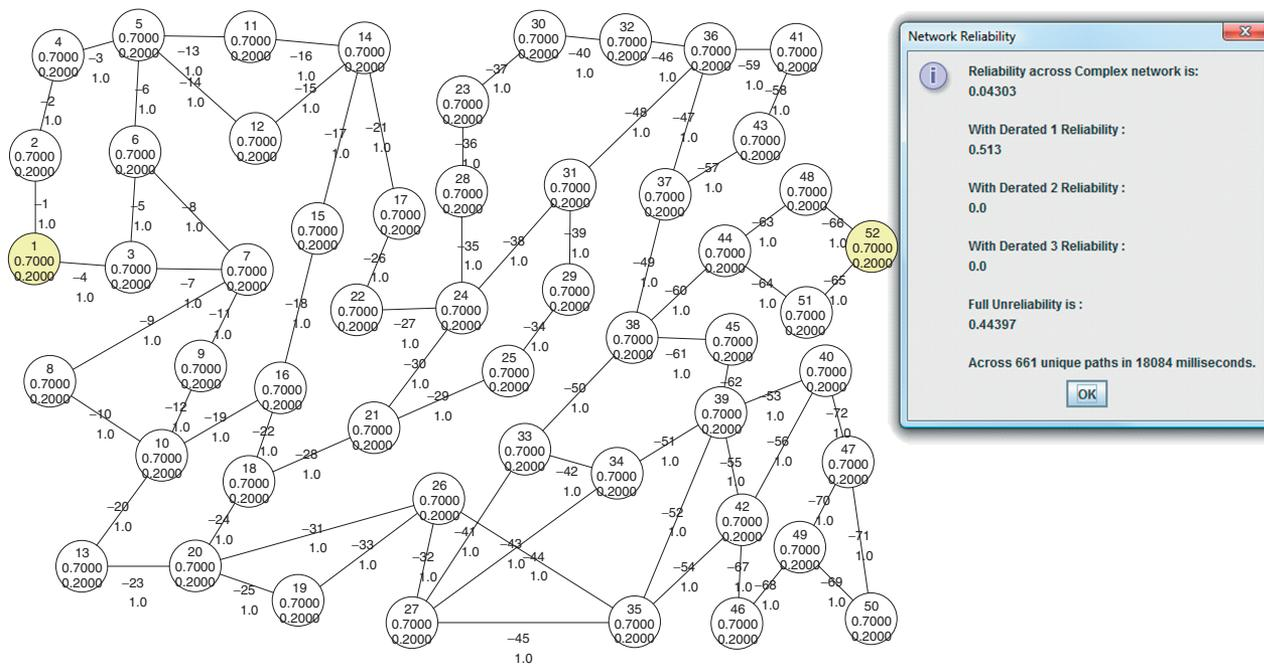
**FIGURE 12** | Example 12: implementation of multistate overlap reliability to 52-node network in 18 s. Solution ( $s = 1, t = 52$ ): full reliability = 0.05, derated reliability = 0.51, full unreliability = 0.44.
