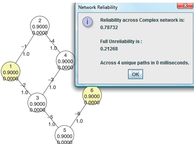
**FIGURE 2** | Example 2: six-node network without including link reliabilities (= 1.0) and (s = 1, t = 6) solution.
