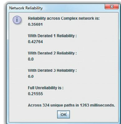
**FIGURE 11** | Example 11: implementation of multistate overlap reliability to 19-node network in 1.26 s. Solution ( $s = 1, t = 19$ ): full reliability = 0.36, derated reliability = 0.43, full unreliability = 0.21.
