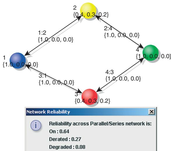
**FIGURE 9** Example 9: active parallel-series system with doubly derated states for 2 and 3.
