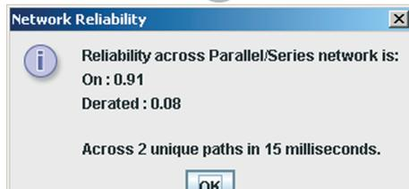
**FIGURE 7** | Example 7: active parallel system with IN(1) and OUT(4) full reliability; others(2,3) are derated.
